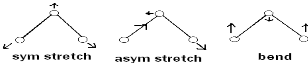
Figure 3.3 The three vibrational modes of water, the symmetric stretch (3656.7, 5160), the asymmetric stretch (3755.8, 5360) and the bending mode (1594.8, 2290) are shown. The vibrational frequencies in \text{cm}^{-1} and the characteristic temperature in K for each mode are shown in parenthesis.
